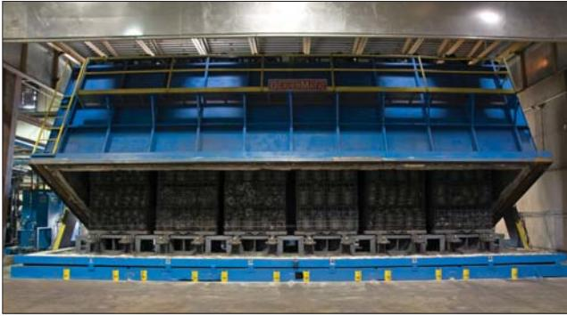
**Fig. 4. Tip-up furnace showing dimensions**
