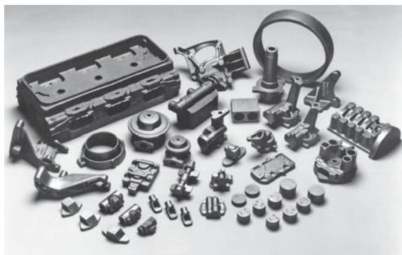
**Fig. 1.** Parts made from gray-iron castings
